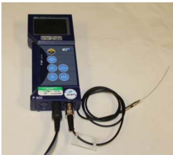
Figure 25. P600 Thermometer and the Type K sensor
