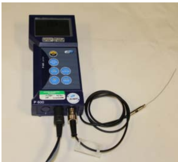
Figure 29. P600 Thermometer and Type K sensor
