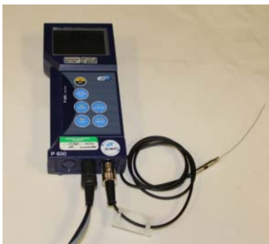
Figure 24. Thermocouple Adaptor and Thermocouple
