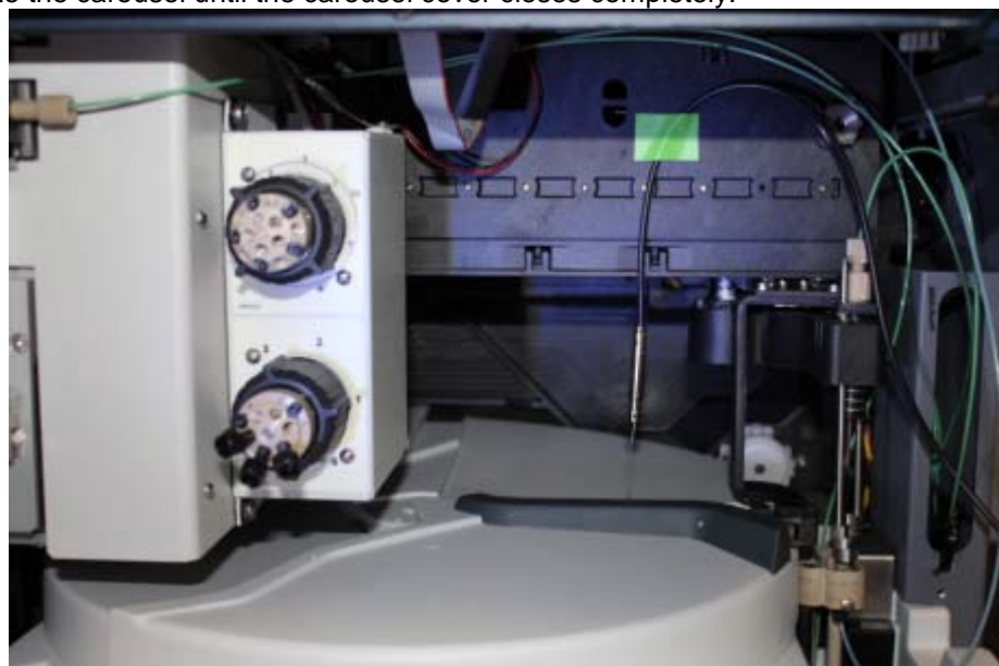
Figure 28. Temperature sensor inserted into the vial
