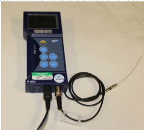
Figure 28. P600 Thermometer and Type K Sensor
