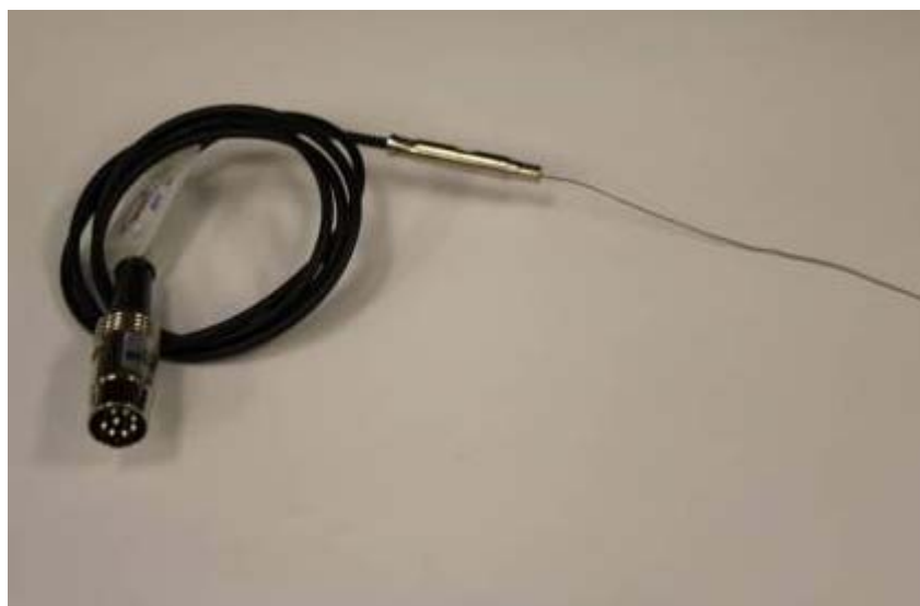
Figure 26. P600 Thermometer and the Type K sensor
