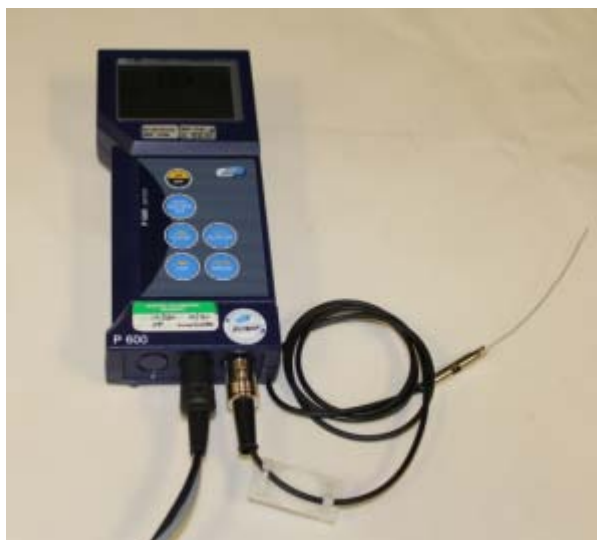
Figure 27. P600 Thermometer and the Type K Sensor
