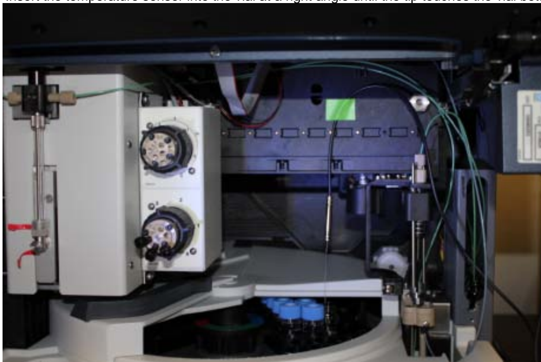
Figure 28. P600 Thermometer with the Type K sensor inserted into the vial
