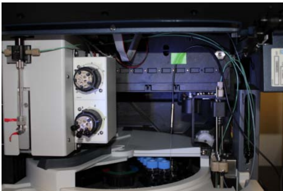
Figure 31. Temperature sensor inserted into the vial
