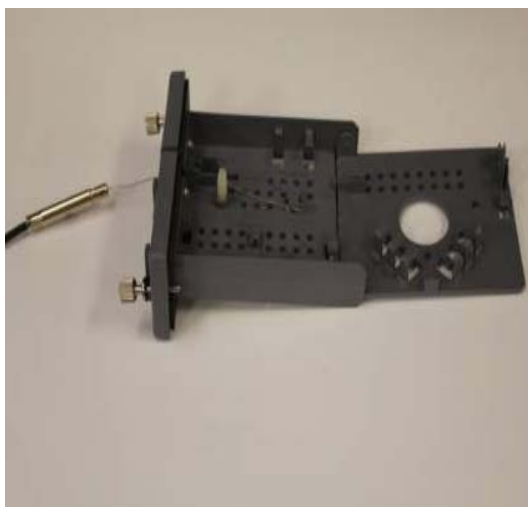
Figure 25. Putting the Thermocouple into the column cartridge
