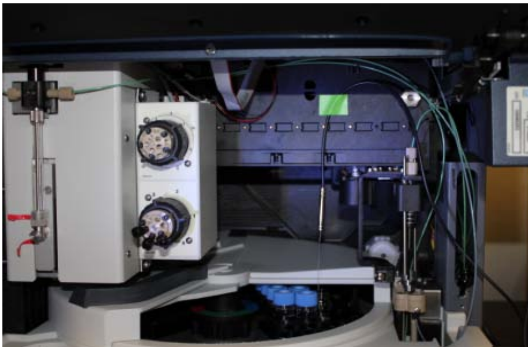
Figure 29. P600 Thermometer with the Type K sensor inserted into the vial
