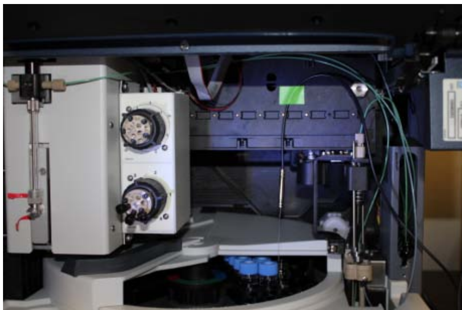
Figure 27. Temperature sensor inserted into the vial
